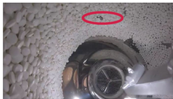
Fig. 7. Maritime BioLogger inside the tablet bed in the ConsiGma® 320 tablet coater
