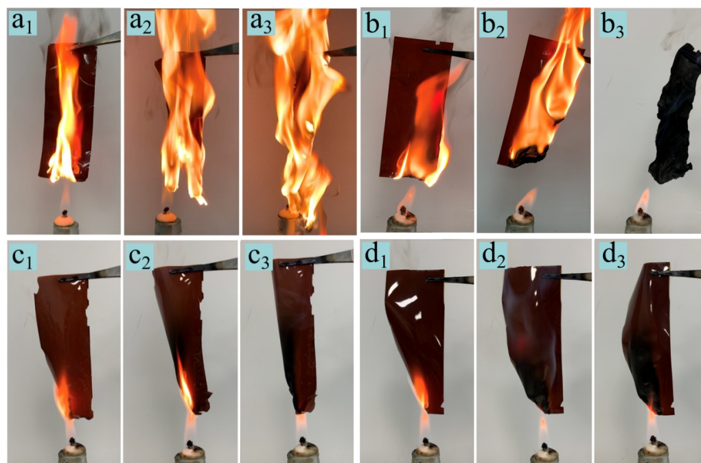
Figure 4. The combustion state of lacquer films with different FR contents in the air: (a) RL, (b) RL/10%IFR, (c) RL/20%IFR, and (d) RL/30%IFR. 1 is the initial state of combustion, 2 is the intermediate state of combustion and 3 is the final state of combustion.
