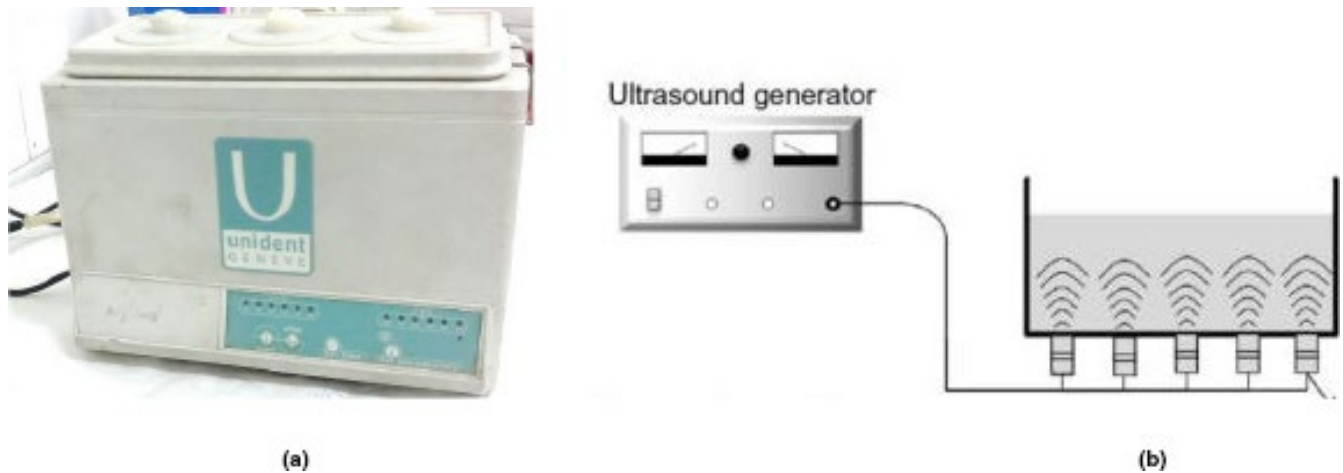
FIGURE 2 (a) Ultrasonic bath apparatus used in this research (b) Schematic view of the apparatus
