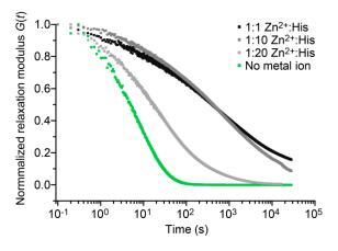
**Figure 6.** Stress relaxation of  $A_{4H3}B_{4H3}$ -containing hydrogels without metal ions and with different  $Zn^{2+}$ :His ratios (1:1, 1:10, and 1:20). The stress relaxation of the hydrogels was monitored after applying a step-strain of 10%.
