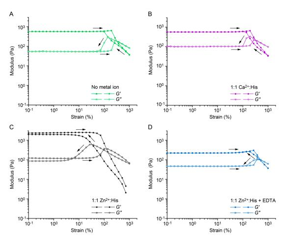
**Figure 3.** Amplitude sweeps of  $A_{4H3}B_{4H3}$ -containing hydrogels in PIPPS buffer. Amplitude sweeps were performed at a constant angular frequency of 10 rad s<sup>-1</sup>, changing the strain amplitude from 0.1% to 1000% and vice versa. (**A**) In the absence of metal ions; (**B**) in the presence of 1:1 Ca<sup>2+</sup>:His; (**C**) 1:1 Zn<sup>2+</sup>:His; (**D**) or 1:1 Zn<sup>2+</sup>:His + 25 mM EDTA (4× excess with respect to the His concentration).
