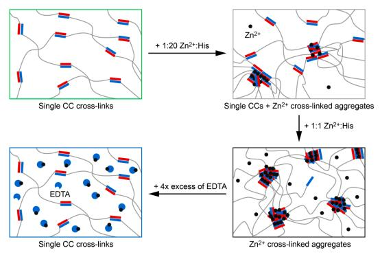
**Figure 7.** Scheme of the cross-linking modes in the hydrogel. In the absence of metal ions, only single coiled coil (CC) cross-links form. At 1:20  $Zn^{2+}$ :His, the hydrogel is cross-linked by a mixture of single CCs and small  $Zn^{2+}$  cross-linked aggregates. At 1:1  $Zn^{2+}$ :His most of the CC-forming peptides participate in these aggregates. The formation of  $Zn^{2+}$  cross-linked aggregates is fully reversible when EDTA is added.
