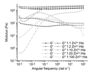
**Figure 5.** Frequency sweeps of  $A_{4H3}B_{4H3}$ -containing hydrogels with different  $Zn^{2+}$ :His ratios. The frequency sweeps were performed from 100 to 0.001 rad s<sup>-1</sup> at a constant strain amplitude of 1%, using  $Zn^{2+}$ :His in ratios of 1:1, 1:2, 1:10, 1:20 and 1:100.
