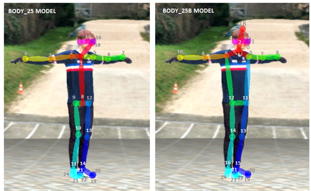
Figure 6. The experimental body_25b OpenPose model is more accurate than the default body_25 one. As an example, the left knee is slightly misplaced on the default model. The keypoint definition differs between both models.
