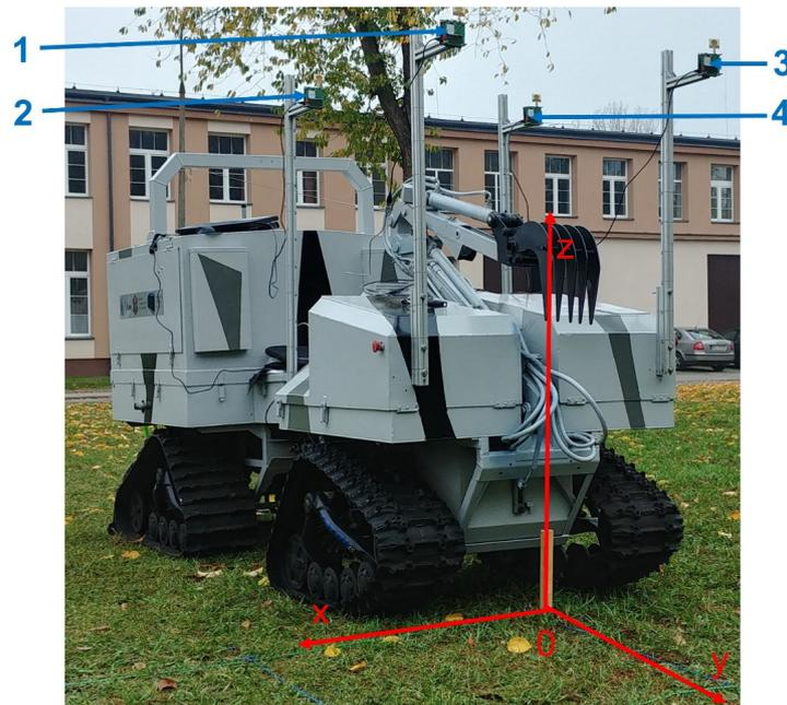
**Figure 6.** The unmanned ground vehicle with the anchors no. 1,2,3,4 and the adopted coordinate system.
