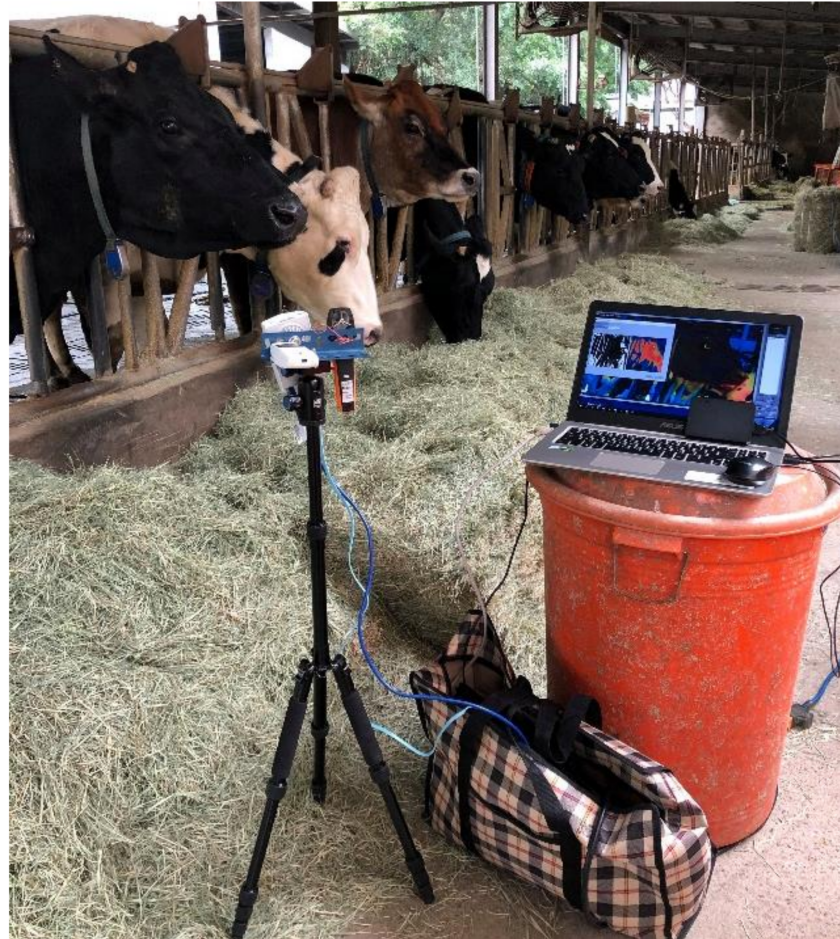
Figure 10. Photography of the experiment for noninvasive cattle body temperature monitoring.
