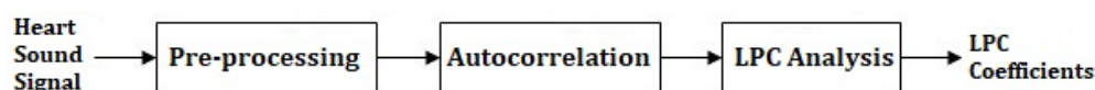
Figure 2. Block diagram for the calculation of the Linear Predictive Coding (LPC) coefficients.
