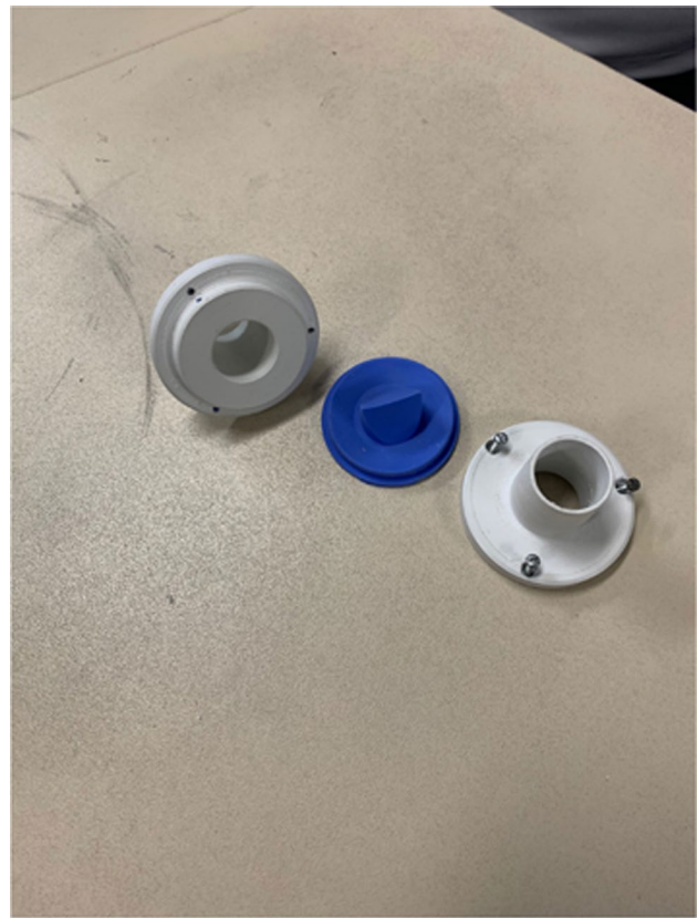
Fig. 13 Two turned parts which can keep the unidirectional valve fitted on the BVM output
