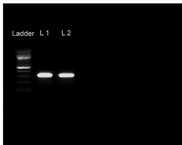
Figure-7: Gel electrophoresis image of the polymerase chain reaction product. L1 - Is the lung from the first calf. L2 - Is the lung from the second calf. The DNA ladder is 100 bp. Mycoplasma bovis band is 319 bp.
