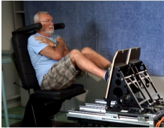
Fig 1. Computer controlled, linear motor powered leg press dynamometer.
