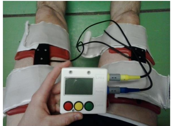
Fig. 3 Surface electrical stimulation: the processing unit and electrodes.
