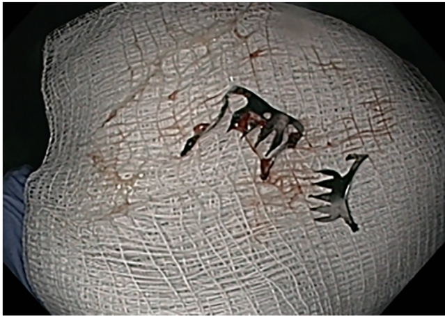
Figure 7. Both ends of the fractured clip after removal.
