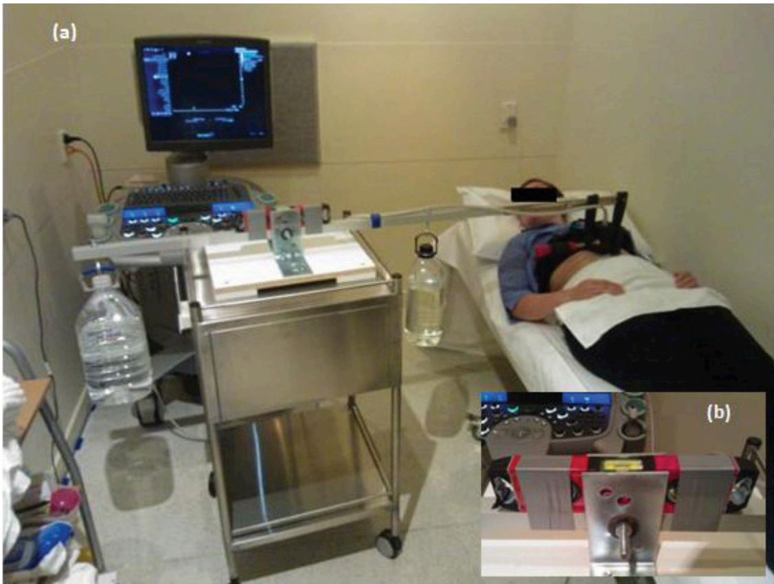
Figure 1: a) A mechanical device used to regulate applied transducer force. b) Spirit level used to ensure cross-bar was horizontal.
