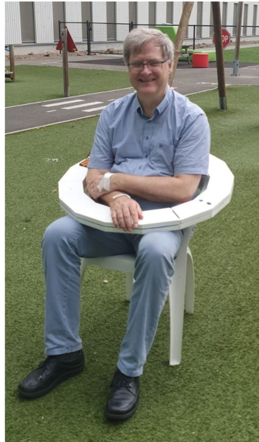
Fig. 2. Photo of the exposure setup. The device is ring-shaped, lightweight, and runs on a battery pack of 10 AA NiMH batteries.
