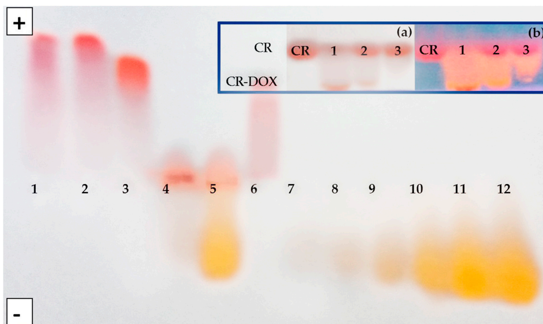
Figure 2. Agarose gel electrophoresis of CR–DOX complexes: (1) CR:DOX = 5:1; (2) CR:DOX = 2:1; (3) CR:DOX = 1:1; (4) CR:DOX = 1:2; (5) CR:DOX = 1:5, and (6) free CR and (7–11) free DOX at increasing concentrations corresponding to the concentration in complexes with CR. Insert: Electrophoresis in 10% polyacrylamide gel: (1) free CR and CR–DOX complexes: (1) CR:DOX = 5:1; (2) CR:DOX = 2:1; (3) CR:DOX = 1:1. It can be seen that CR–DOX complexes migrated faster than free CR. (a) visible light; (b) UV light (DOX better visible).
