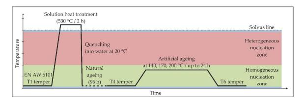
Figure 2. Temperature-time scheme of the conventional heat treatment procedure to the T6 temper.
