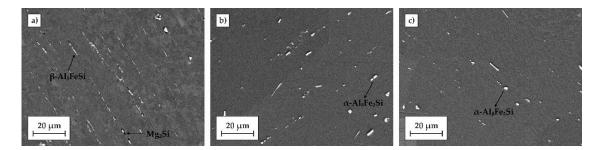
**Figure 7.** SEM micrographs of longitudinal sections of the wire rod after different heat treatment stages: (a) as-fabricated; (b) solution heat treated at 530 °C/2 h, water quenched, naturally aged, artificially aged at 170 °C/24 h; (c) solution heat treated at 530 °C/2 h, cooled down by flowing air forced to 170 °C, artificially aged at 170 °C/24 h.
