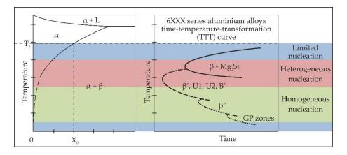
Figure 1. Scheme of the precipitation kinetics in 6xxx series alloys.
