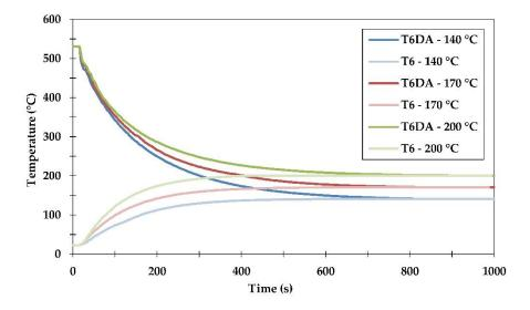
**Figure 4.** Temperature evolution measured during alloy quenching from a solutionizing temperature of 530 °C directly to artificial ageing temperatures of 140 °C, 170 °C and 200 °C (T6DA procedure), as well as during heating to artificial ageing temperatures from room temperature (T6 temper procedure).
