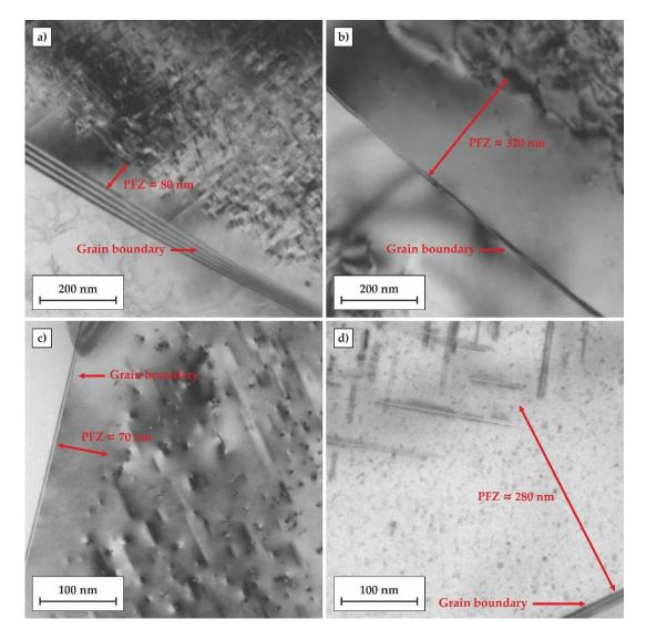
**Figure 9.** TEM micrographs showing grain boundary regions of the alloy after two investigated heat treatments: (**a**,**c**) conventional heat treatment to the T6 temper including artificial ageing at 170 °C for 24 h; (**b**,**d**) quenched directly to the temperature of 170 °C followed by 24 h artificial ageing (T6DA). PFZ, precipitate-free zones.
