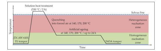
Figure 3. Temperature-time scheme of the direct ageing procedure (T6DA).
