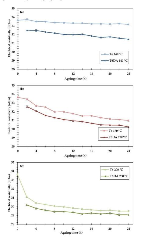
**Figure 6.** Electrical resistivity of the EN AW 6101 wire rod subjected to artificial ageing at (**a**) 140 °C, (**b**) 170 °C and (**c**) 200 °C, using two different heat treatment procedures: to the conventional T6 temper and directly to the ageing temperature.
