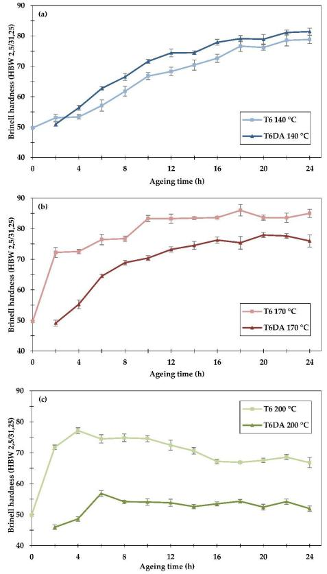
**Figure 5.** Brinell hardness (HBW 2.5/31.25) of the samples subjected to artificial ageing at (**a**) 140 °C, (**b**) 170 °C and (**c**) 200 °C, using two different heat treatment procedures: to the conventional T6 temper and directly to the ageing temperature.
