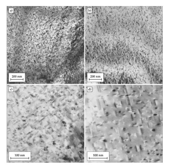
**Figure 8.** TEM micrographs showing the matrix precipitation of the alloy after two investigated heat treatment procedures: (**a**,**c**) conventional heat treatment to the T6 temper including artificial ageing at 170°C for 24 h; (**b**,**d**) quenched directly to the temperature of 170 °C followed by 24 h of artificial ageing (T6DA).
