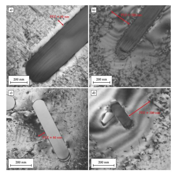
**Figure 10.** TEM micrographs showing second phase particle regions of the alloy after two investigated heat treatments: (**a**,**c**) conventional heat treatment to the T6 temper including artificial ageing at 170 °C for 24 h; (**b**,**d**) quenched directly to the temperature of 170 °C followed by 24 h of artificial ageing (T6DA).
