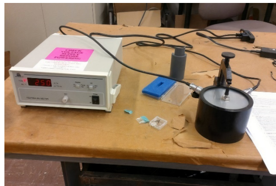
Figure 10. d_{33} Meter showing calibration block force reading [14].
