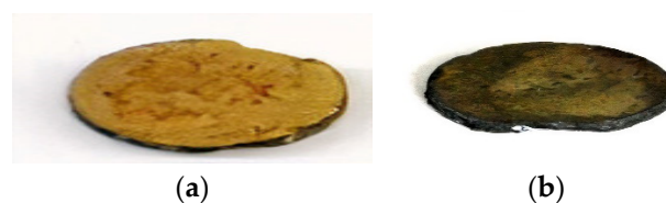
Figure 15. Bismuth titanate (BiTi) drop-in wafers. To the left in (a) is the pre-irradiated image and to the right in (b) is the post-irradiated bismuth titanate (BiTi) sample [14].
