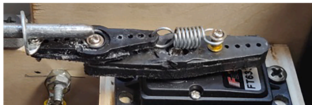
Fig. 21. Closeup of servo arm showing #10 washer (bent and drilled) on end of lever arm and small tension spring. The remainder of parts (plastic arms, screws, and grommets) are from the servo package. This flexible arm accommodates the occasional misalignment of the bolt head and socket. If the socket cannot slide into position easily, the spring allows the servo arm to rotate anyway. As the drive motor turns, the socket will eventually slide onto the bolt head.
