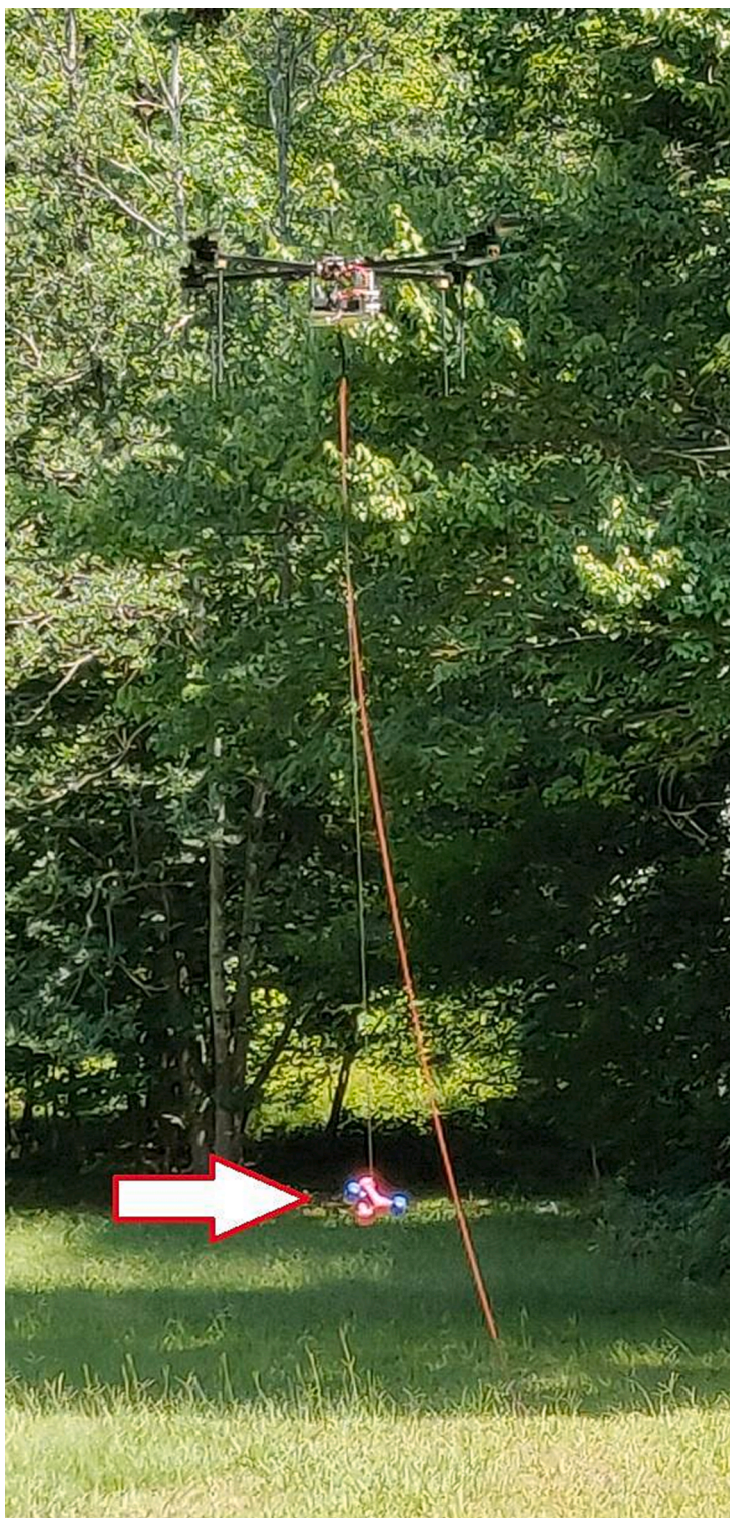
Fig. 29. Tether powered UAV lifting bundle of hand weights for payload vs power measurement.
