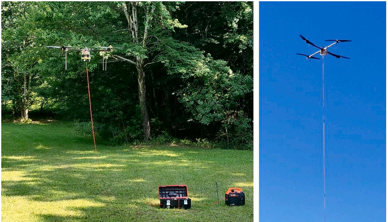
Fig. 28. Initial takeoff with excess cable extended from spool and gathered on ground (left). Climb out with UAV pulling tether from freewheeling spool (right).
