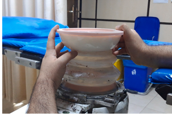
Fig. 2. Placement of the raw milk sample package on the electromagnetic shock wave generator.
