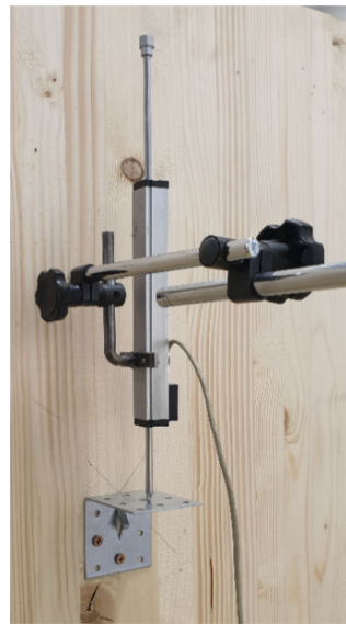
Figure 4. Displacement tracer—sensor from company Ahlborn [42].
