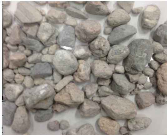
Figure 6. Aggregate morphology after ball milling.
