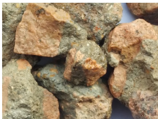
Figure 3. Appearance of the recycled coarse aggregate and attached mortar.
