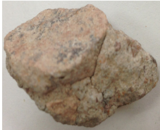
Figure 5. Aggregate morphology after calcination.
