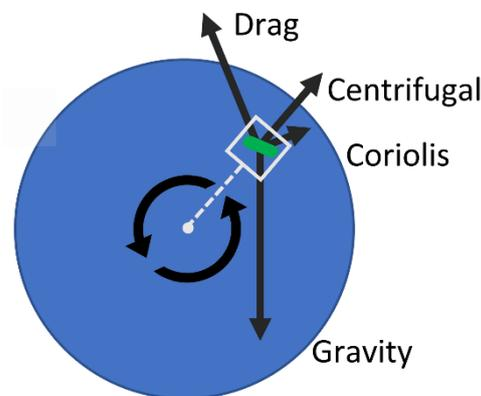
**Figure 3.** Free body diagram of a particle immersed in an RWV. Acceleration terms are described in Equation (3). The simulation domain is a rectangular box in a rotating reference frame.
