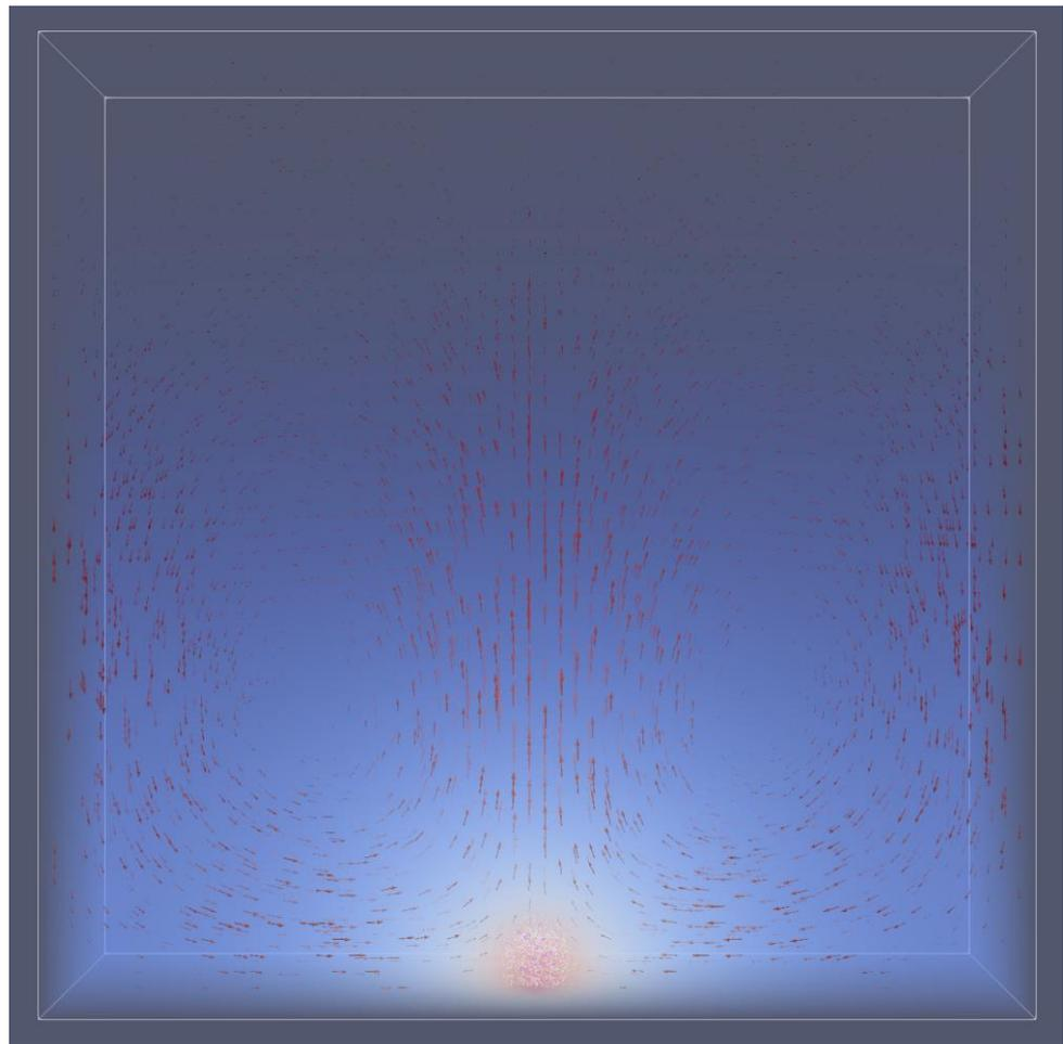
**Figure 10.** Natural Convective Flow. A spherical biofilm placed on the simulation floor exhibited solute convective flows in a 1 g gravity condition. Red velocity arrows, in units of  $s^{-1}$ , are scaled up by  $1000\times$ . The concentration field of acetate is depicted from high to low as red to blue. Fluid simulation boundaries are periodic except on the floor and ceiling of the box.
