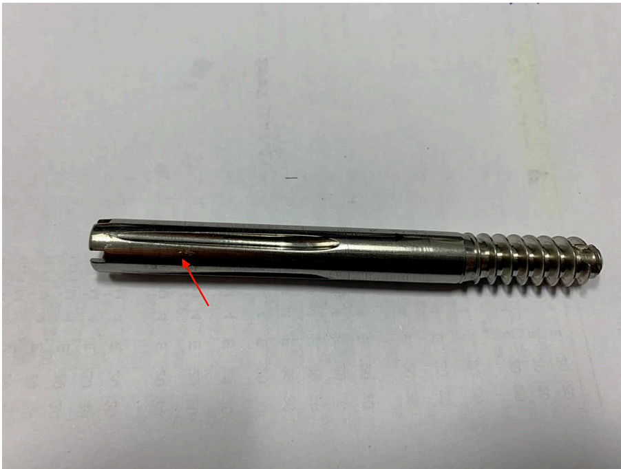
Fig. 3. Macroscopic image of the removed lag screw (A). The red arrow demonstrates the defect, caused by the set screw deviated from the groove (B).
