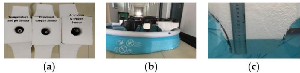
Figure 19. Floating structure test diagram of a floating UAV: (a) sensor installation diagram; (b) inflatable pool test; and (c) sinking depth of the floating structure.
