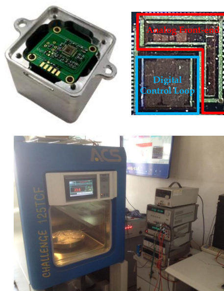
Figure 12. The interface integrated circuit and test system of the DRG.
