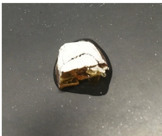
Fig. 11. Amorphous IND exposed to water and a drop of ISO for 2 min.
