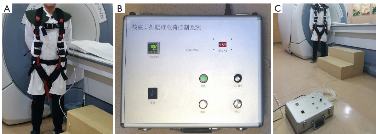
Figure 1 The axial loading MRI device consists of wearable components and pressure components (A,B). Pressure is applied in the pneumatic mode by the control system, which was placed as far away from the magnet as possible (C). MRI, magnetic resonance imaging.
