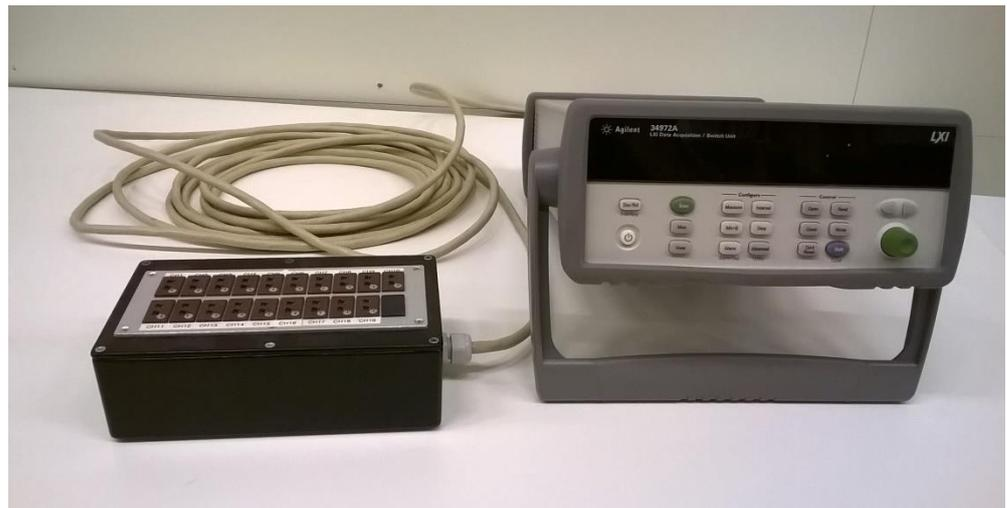
**Figure 3.** The data logger along with the reference junction box. The thermocouples are connected to the miniature thermocouple sockets at the top of the box. The cable from the box connects to the data logger DC voltage input channels.
