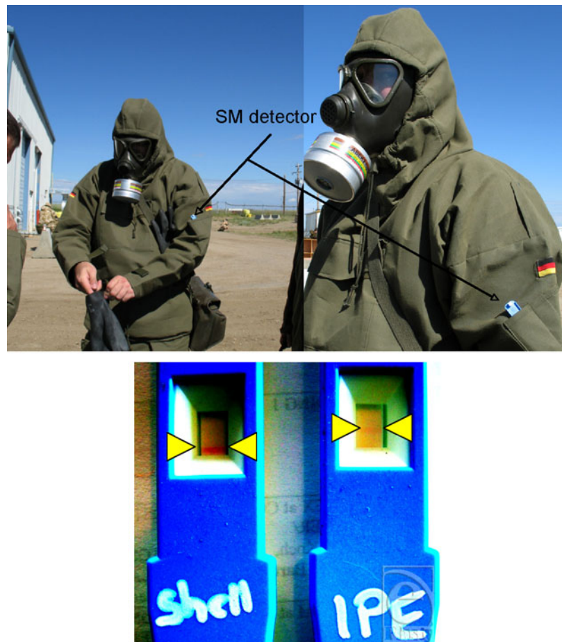
Figure 2. Sulfur mustard detector was used to detect environmental traces of sulfur mustard. Sulfur mustard detector was attached to an individual protective equipment before the soldier entered a cave with an open sulfur mustard grenade shell. Sulfur mustard detector was held over the shell for 5 seconds. After leaving the cave, the sulfur mustard detector showed red lines as positive results for the individual protective equipment as well as for the shell.
