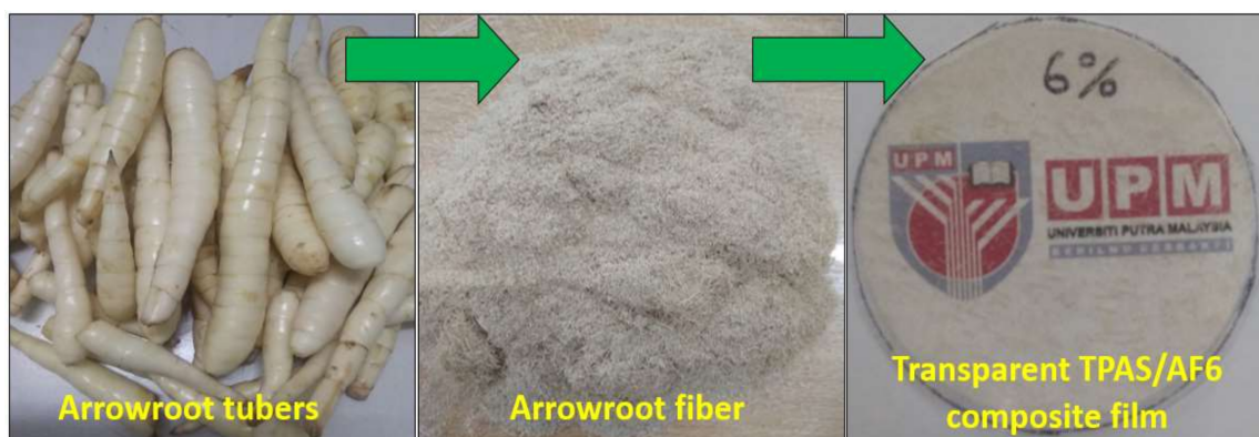
Figure 1. The arrowroot tubers, the fiber obtained from starch extraction, and transparent TPAS/AF composite film with 6% fiber loading.
