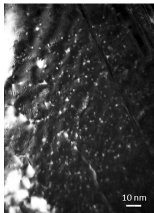
Figure 1. Stacking fault tetrahedra formed in Cu. The sample was deformed at room temperature with a strain rate of 10^6/s . Dark-field weak-beam TEM observation along [110] direction.
