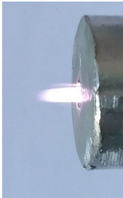
Figure 4. Plasma jet during normal operation. Experimental conditions: U_i = 400 \text{ V}_{rms} , R_{b2} = 20 \text{ k}\Omega , Ar as carrier gas at flow rate of 3 LPM.
