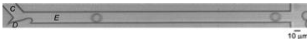
Figure 1. Image of the Y-junction microfluidic device showing the continuous phase channel (C), the dispersed phase channel (D) and the emulsion channel (E) (Figure reproduced by permission of John Wiley and Sons [license number 2711390361304]).
