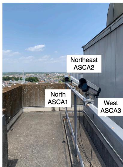
Fig. 1. The cameras of ASCA installed on the roof of the Sagamihara campus, Aoyama Gakuin University, Japan.
