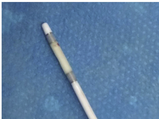
Fig. 5. After filling, the balloon was attached to the catheter wall.
