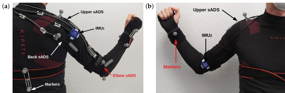
Figure 3. Location of sensors on the compression jacket. (a) Back view. The reflective markers are shown in bright grey, the IMU 1 and the two sADS on the shoulder (upper and back) and the sADS on the elbow. (b) Front view, which shows two reflective markers and the IMU 2 .
