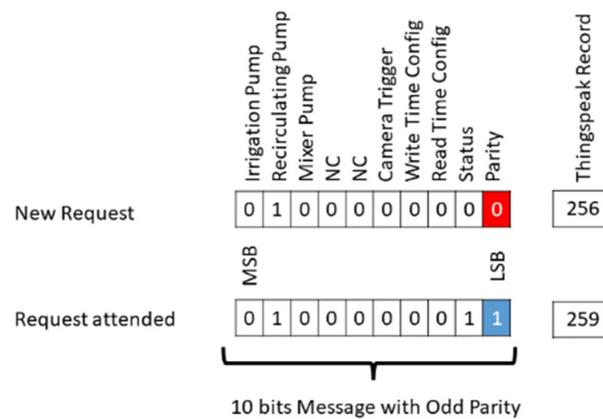
**Figure 5.** Command vector for remote operation from App.
