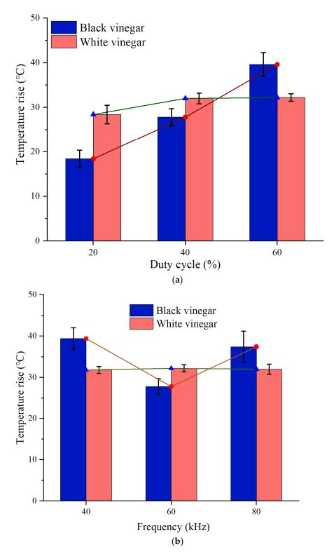
**Figure 6.** (a) Effect of different duty cycle on the temperature rise; (b) effect of different frequency on the temperature rise.
