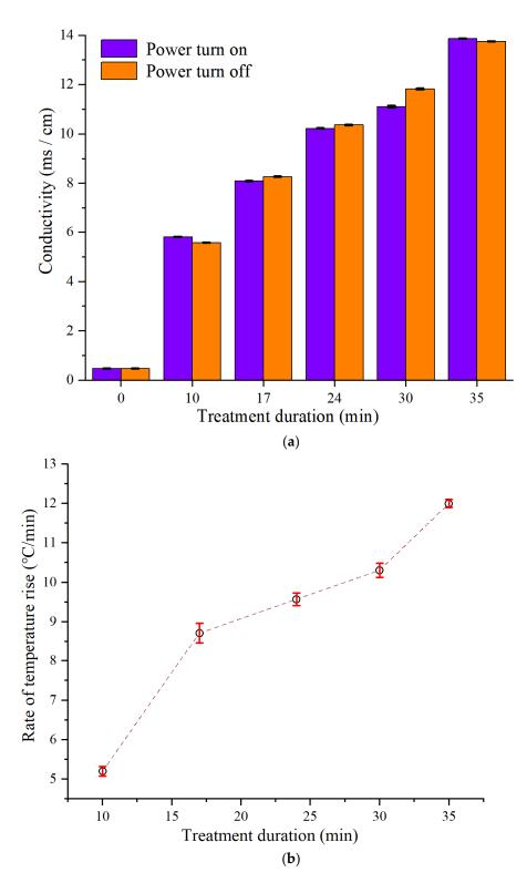
**Figure 4.** (a) Effect of the treatment duration on the sample conductivity; (b) Effect of the treatment duration on the temperature rise.
