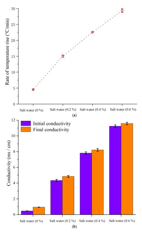
**Figure 5.** (a) Effect of NaCl solutions on the temperature rise; (b) effect of NaCl solutions on the conductivity.
