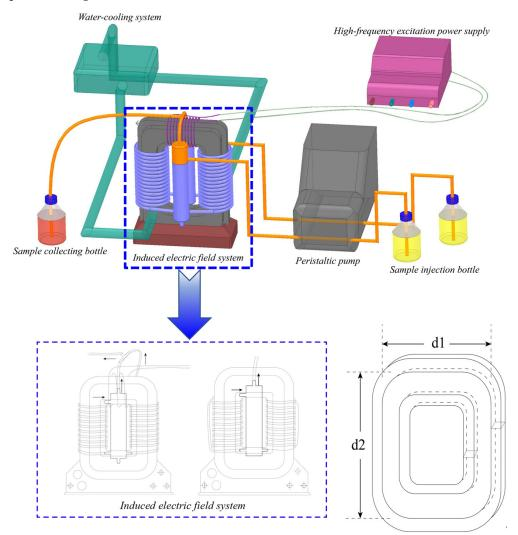
**Figure 3.** The schematic diagram and flow chart of the induced electric field heating unit (d1 = 15 cm, d2 = 25 cm).
