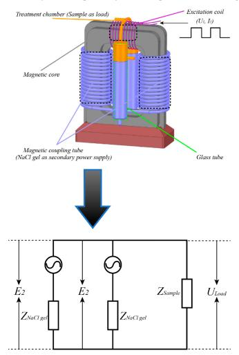
Figure 2. The schematic diagram of the induced electric field heating system and its equivalent circuit.
