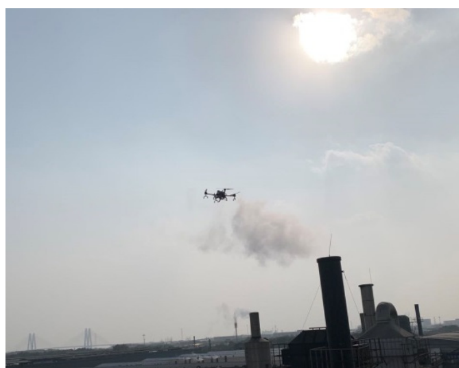
Figure 3. On-situ photograph of PM measurement from the chimney by a self-developed PM detector on an UAV.
