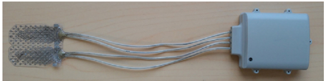
FIGURE 1: ECoGI-64D - the picture shows the subdural grid, connecting cables and a wireless case
