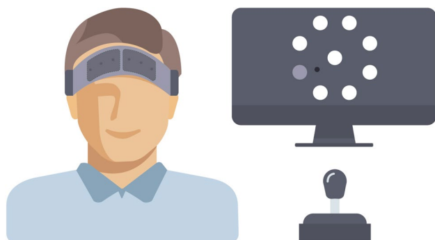
Fig. 1 Schematic depiction of the placement of the two fNIRS sensor pads (left) above the eyebrows with the inside of both sensor pads aligned with the nasion and the learning task (right) with the joystick mounted on the table and the task presented on the monitor (cursor in black, the eight targets spaced at an equal distance from the middle with one selected target being darker)
