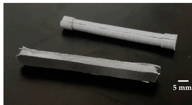
Figure 1. Picture of the composites: Cylindrical for Villari measurements and rectangular prims for measurements of microindentation.
