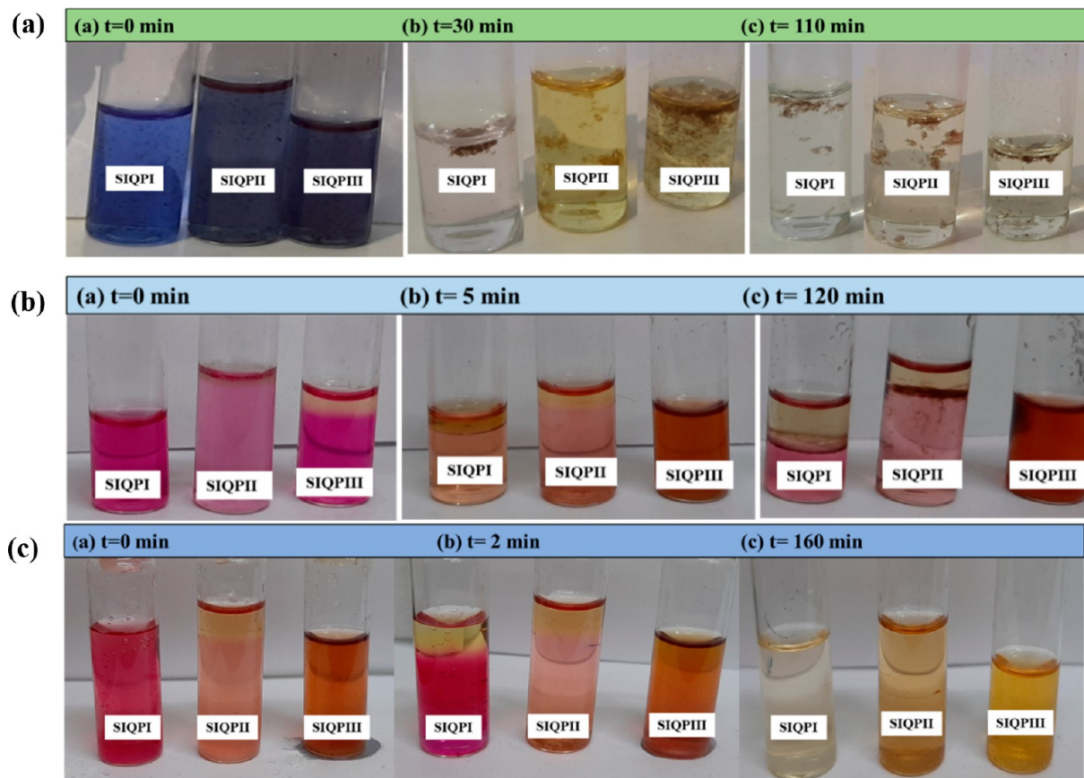
Figure 4. (a) MB PCR by 0.01 mmol of SIQPI, II, and III with GO in aq-ACN at (a) t = 0 min, (b) 30 min, and (c) 110 min under SL. (b) QHIn PCR by 0.01 mmol of SIQPI, II, and III with GO in aq-ACN-EtOH at (a) t = 0 min, (b) 5 min, and (c) 120 min under SL. (c) QHIn PCR by 0.01 mmol of SIQPI, II, and III with NaCl in mixed solvent at (a) t = 0 min, (b) 2 min, and (c) 160 min under SL.
