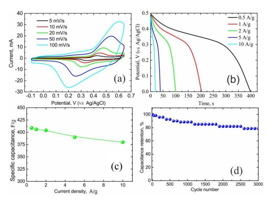
**Figure 6.** Electrochemical performance of NiO/C nanocomposite (60 wt% NiO) in a three-electrode cell in a 1 M KOH aqueous solution: (a) CVs at various scan rates; (b) galvanostatic discharge curves at various current densities; (c) specific capacitance as a function of current density; (d) cycling stability at the current density of 2 A/g.
