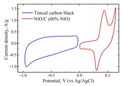
**Figure 8.** CV curves of carbon black Timcal Super C65 (CB) and NiO/C (60 wt% NiO) in a three-electrode cell in a 6 M KOH solution at a scan rate of 50 mV  $\rm s^{-1}$ .
