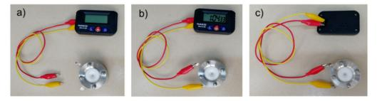
**Figure 10.** Application of the asymmetrical two-electrode assembled cell (NiO/C (60 wt% NiO) as a positive electrode and CB Timcal Super C65 as a negative electrode) in a 6 M KOH aqueous solution: (a) photograph of an asymmetrical two-electrode assembled cell charged at 0.5 mA and a battery-free quartz clock; (b) photograph of a quartz clock (front side) in the process of charging; (c) photograph of a quartz clock (back side) in the process of charging.
