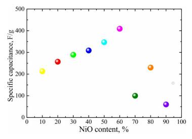
**Figure 5.** Specific capacitance as a function of NiO content in NiO/C composites at a current density of  $0.5 \text{ F g}^{-1}$  in a three-electrode cell in a 1 M KOH solution. The results are divided into two groups.
