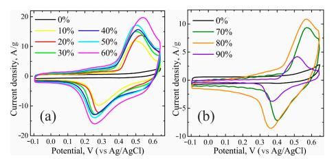
**Figure 4.** Cyclic voltammograms (CVs) of NiO/C samples, divided into two groups with NiO concentrations of: (a): 0, 10, 20, 30, 40, 50, 60 wt%; (b) 0, 70, 80, 90 wt%.
