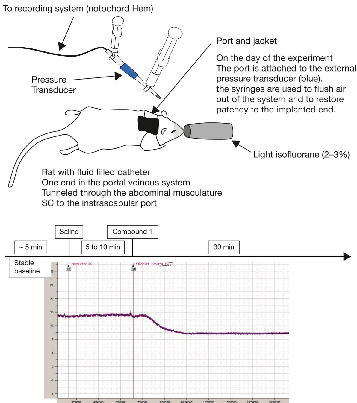
Fig. 1. Experimental set-up.
