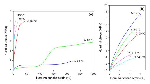
**Figure 4.** Nominal stress–nominal strain curves obtained in uniaxial tensile tests at temperatures indicated. (**a**) amorphous samples, A; (**b**) cold crystallized samples, CC. Note the different scale on the stress and strain axes in (**a**,**b**).
