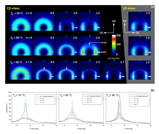
Figure 12. (a) Transmission 2D-WAXS patterns of the initially amorphous A samples deformed in the plane-strain compression
