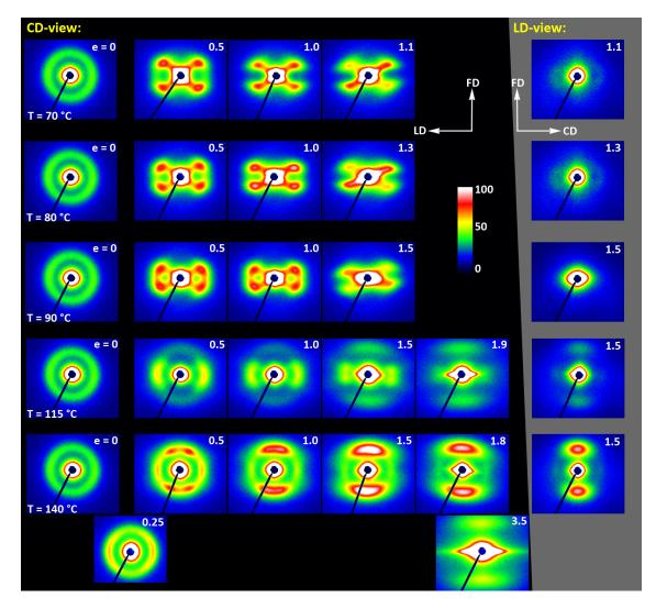
**Figure 17.** 2D-SAXS patterns of the initially amorphous A samples deformed in the plane-strain compression at temperature  $T_d = 70-90$  °C (**rows from top to bottom**), to the indicated true strain. The patterns on the left (black background) were obtained in the CD-view. The patterns in the column on the right (gray background) are LD-view.
