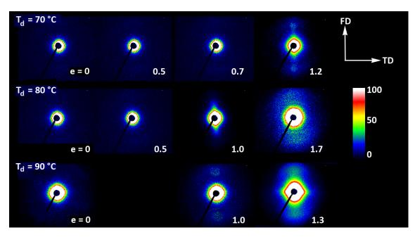
**Figure 11.** 2D-SAXS patterns of the initially amorphous A samples deformed in uniaxial tension at temperature  $T_d = 70 \degree C$  (**top row**),  $T_d = 80 \degree C$  (**middle row**), and  $T_d = 90 \degree C$  (**bottom row**). The true strain indicated for each pattern is the local true strain calculated from the distance of the ink marks printed on the sample.
