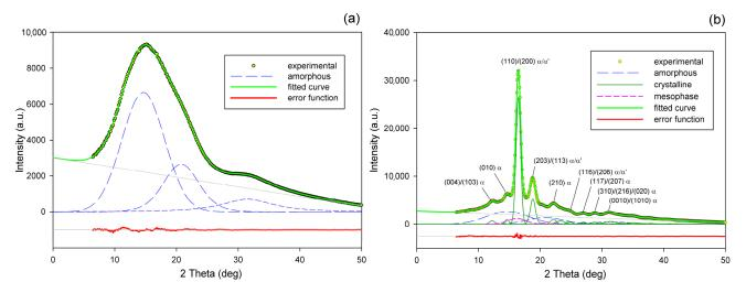
**Figure 2.** Examples of fitting the amorphous halos and mesomorphic and crystalline peaks to the scattering curve of A (**a**) and CC samples (**b**).
