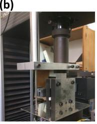
Figure 1. Schematic drawing (a) and a photograph (b) of the channel-die compression fixture.
