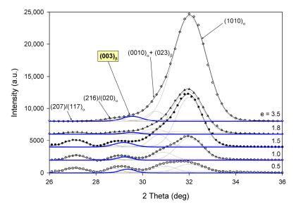
At the lower deformation temperature, the  $\beta$  peak was hardly detected, which indicates that  $\alpha \rightarrow \beta$  transformation was most probably not active then.
