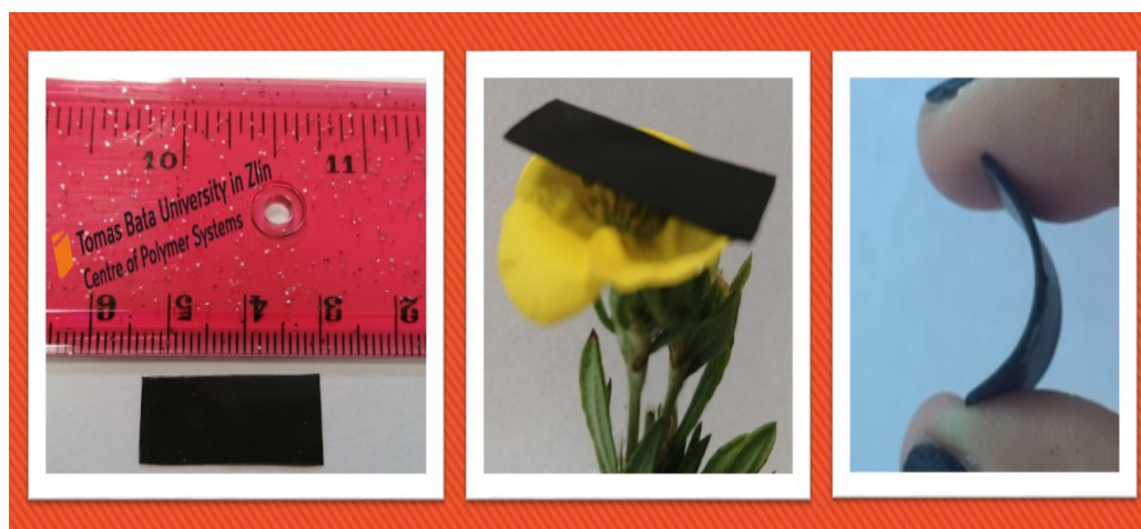
Figure 3. Digital photograph of PP nanocomposite embedded with \text{MnFe}_2\text{O}_4 spinel ferrite nanoparticles and reduced graphene oxide (RGO) as nanofillers.
