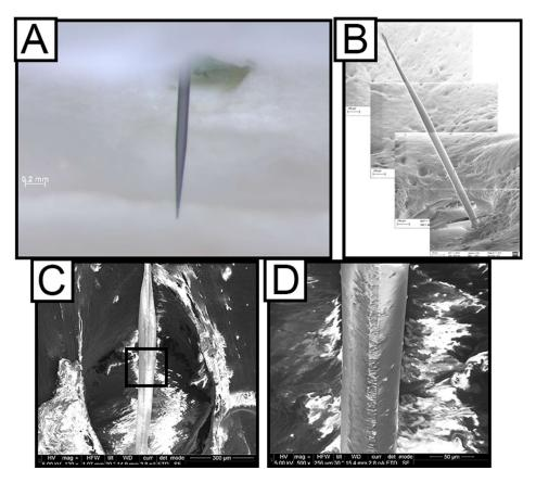
**Figure 3.** Ex vivo Characterization of coating stability. Dip-coated probes inside the skull with all tissue removed captured using optical microscopy (**A**) and SEM (**B**) showing that the SMP coating of the silicon shanks is still intact after two weeks. (**C**) Side-view SEM image of a dip-coated probe, explanted after 16 weeks in the rat cortex, showing the SMP coating intact. Black rectangle inset is blown up further in (**D**).
