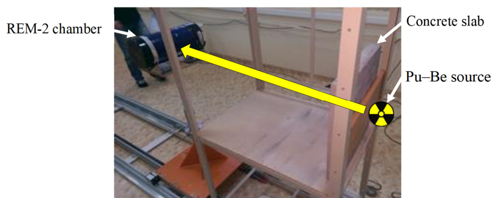
Figure 4. Experimental stand for measurements of neutron radiation shielding efficiency [28].
