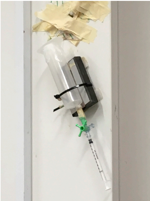
Figure 11. Sample catcher used to receive the hyperpolarized [ 1\text{-}^{13}\text{C} ]pyruvate solution
